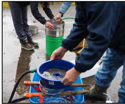
A sieving process and vortex method are used to separate eggs from the beach sediment.
